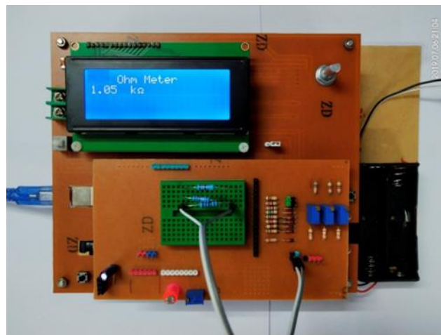
Figure 8: Photograph of measuring results for resistance circuit
