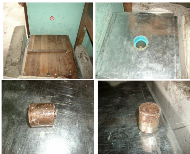
Figure 3. Am-Be Neutron Source for Irradiation Facility with 550 mCi
