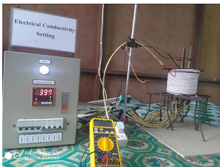
Figure 6 Experimental set-up of resistivity measurement
