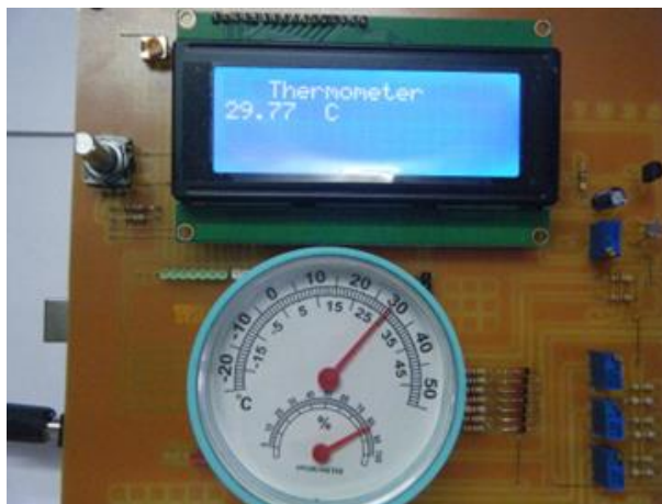
Figure 10: Photograph of measuring results for temperature
