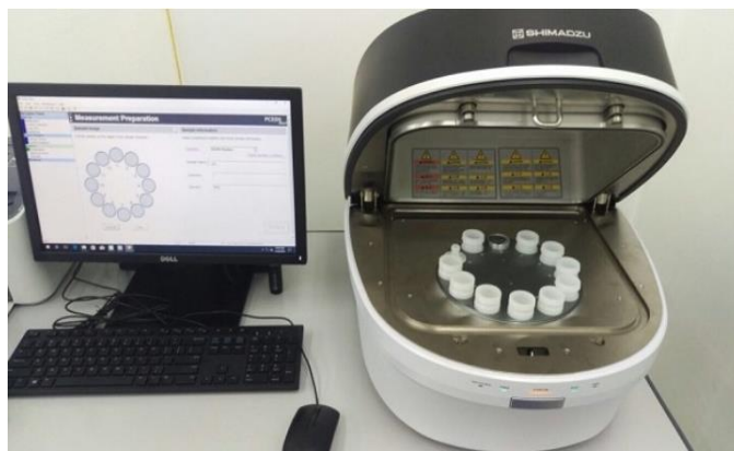
Figure 13 Measurement condition of Energy Dispersive X-Ray Fluorescence (EDXRF) Spectrometer (EDX 7000 Shimadzu)
