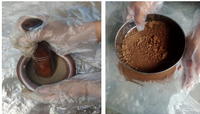
Figure 2 Photographs of grinding by mortar and sieving by 0.01cm sieve
